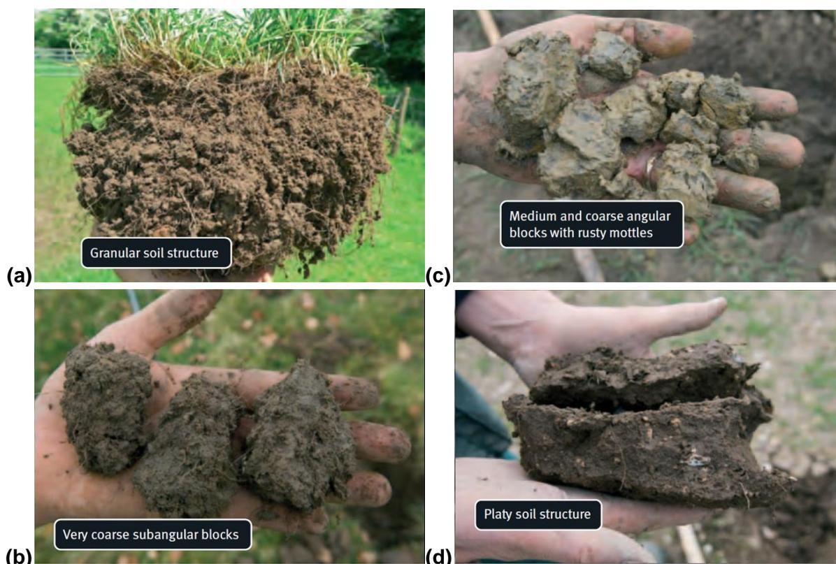
**Fig.1.** Photographs of soils showing common structural characteristics
