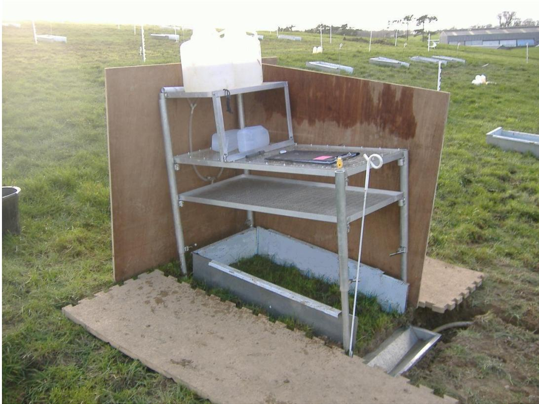
**Figure 3.3:** Rainfall simulation apparatus used to generate overland flow during Experiments 1 and 2
