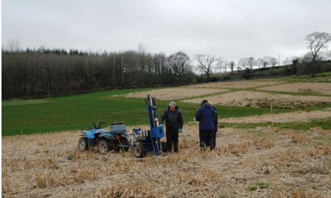
Soil CO<sub>2</sub> flux system used to measure CO<sub>2</sub> concentration (Hillsborough, 2013).
