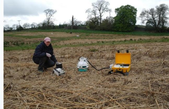
Carbon flux estimation using Eddy Covariance. Measures total ecosystem fluxes of carbon (Hillsborough, 2013).
