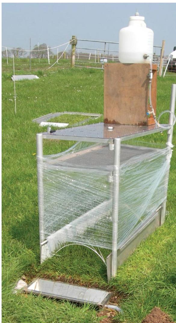
*Rainfall simulator, showing tray inserted into the soil at the bottom of the plot to collect surface runoff*
